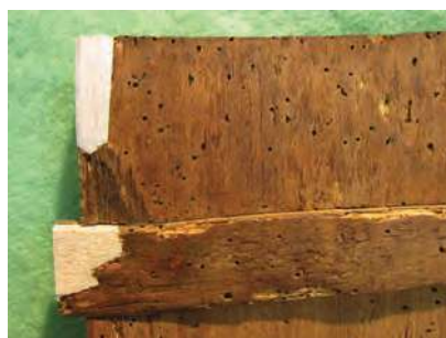
▲ Fig. 19. Crossbar lacuna filled with new wood.
