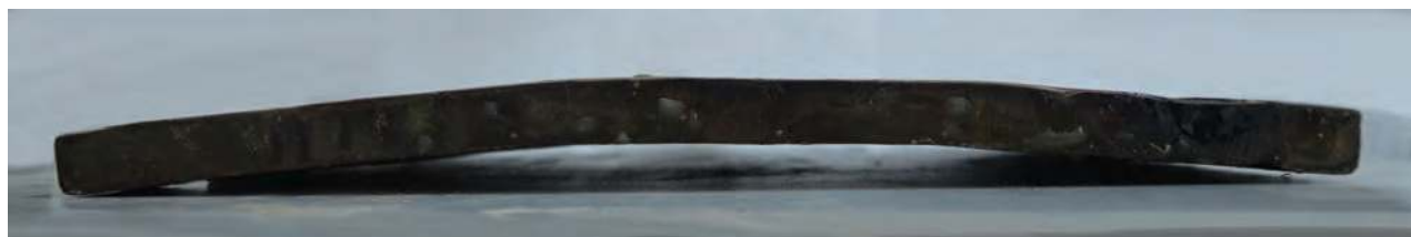
◆ Fig. 4. Icons showing bowed / cupped panels (concave to the unpainted surface): a-b) drawings by Dumitrița-Daniela Filip, c) the wood panels of the Christ Pantokrator with Scenes and Saints (cat. 19), d) Mother of God Smolenskaya (cat. 8), e) Resurrection of Christ / Descent into Hell, with Passion and Feasts (cat. 30), f) Mother of God Feodorovskaya (cat. 7), g) Christ Pantokrator (cat. 20), h) Mother of God Akhtyrskaya (cat. 17), i) Resurrection of Christ / Descent into Hell and Twelve Feasts (cat. 31), j) Four-part Icon (cat. 48), k) Saint Nicholas of Myra (cat. 37a), l) Mother of God Assistant in Childbirth (cat. 12), m) Four-part Icon (cat. 46), and n) Mother of God Seeker of the Lost (cat. 5) icons.
