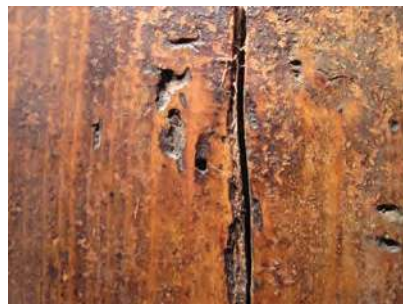
▼ Fig. 4. Crack in the central longitudinal area of the panel.
